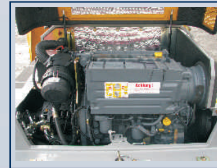
Optimum maintenance conditions and few downtimes ensured by good accessibility to the drive unit and to the hydraulic components.
