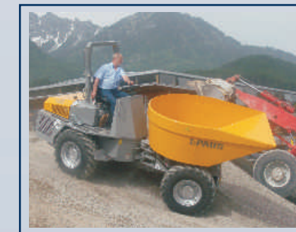
High degree of operating safety is achieved by DSC, which protects the dumpers from exceeding the permissible speed in downhill runs.
