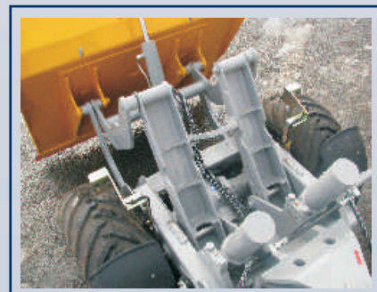
Extraordinary powerful and productive dumper series SMK due to innovative kinematics in connection with two lifting cylinders.
