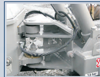
Extreme manoeuvrability and off-road mobility due to 3-point articulated-pendulum joint.
