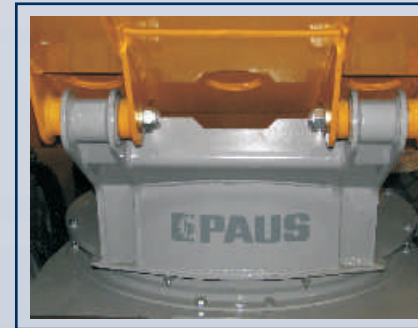
Extraordinary durability of the dumpers guaranteed by the heavy-duty rotary joint equipped with two double-acting swivel cylinders.
