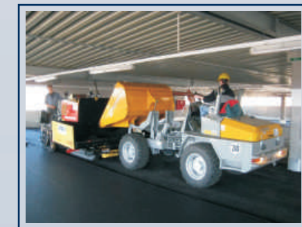
Low vehicle height is achieved by the movable safety guard (e.g. in underground car parks).
