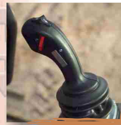
Electro-hydraulic anticipatory control via multifunctional joystick
