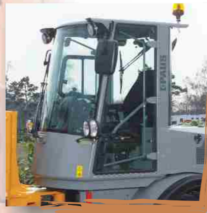
Plain entrance on both sides, control device foldable to the back, ergonomically designed joystick, orthopaedic comfortable seat with safety belt and disc support
