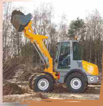
Z-kinematics: two lifting cylinders provide high lifting forces during operation of bucket
