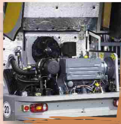
Extremely good accessibility for inspection and maintenance works due to the GFK engine cover that can be opened widely
