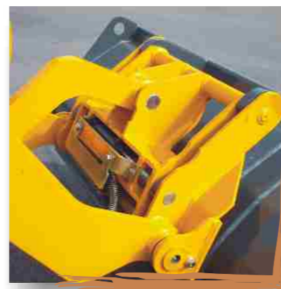
A PAUS standard: hydraulic quick-change device for many attachments
