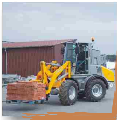
Excellent payload during operation as a forklift combined with an optimum parallel guidance
