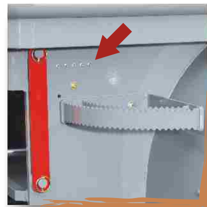
The central bar close to the steps allows easy lubrication of the complete caisson
