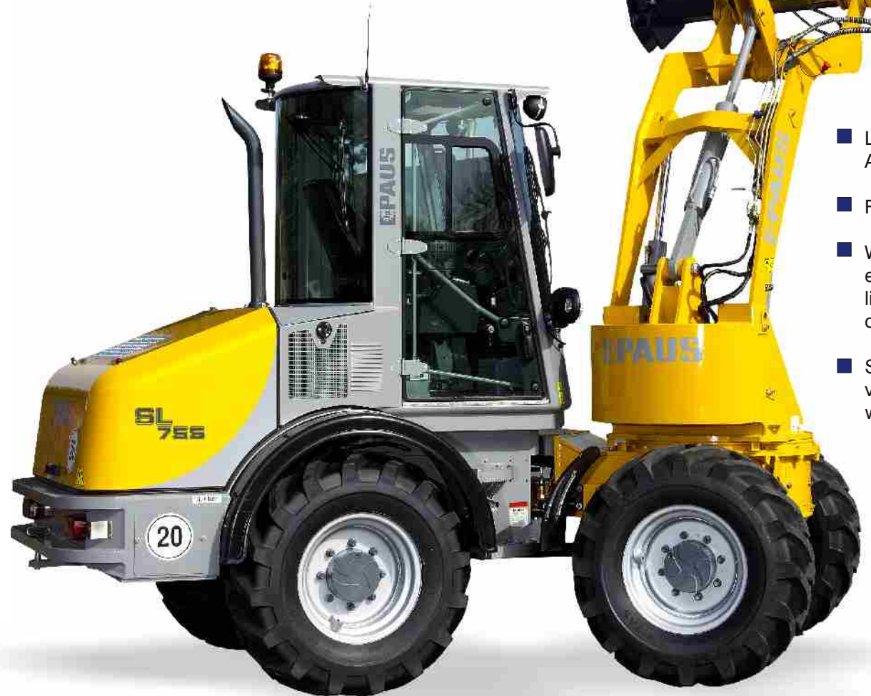
Lowering cut-off automatics avoids damage to the tires in swivelled position
