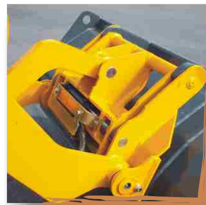
A PAUS standard: hydraulic quick-change device for many attachments
