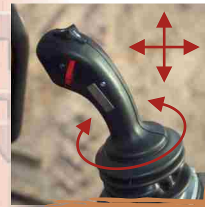
Electro-hydraulic anticipatory control via multifunctional joystick; swivelling function by turning the joystick
