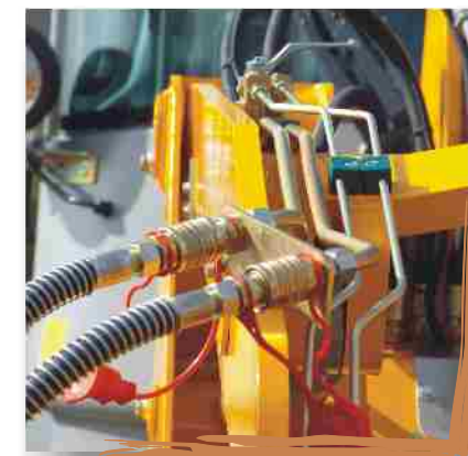
Additional connection for hydraulic attachments, e.g. concrete-mixing bucket or power sweeper
