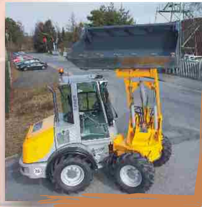
Swivelling device with two directly actuated cylinders, for long-term smooth working at highest degree of operating safety
