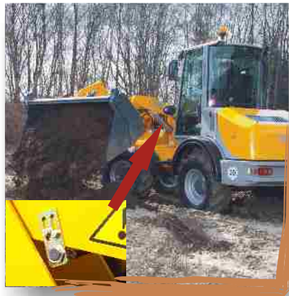
Lowering cut-off automatics avoids damage to the tires in swivelled position
