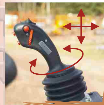
Electro-hydraulic anticipatory control via multifunctional joystick: For TSL 855: swivelling function by turning the joystick
