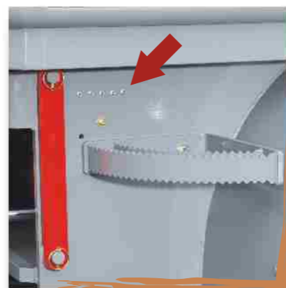
The central bar close to the steps allows easy lubrication of the complete chassis
