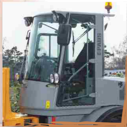
Plain entrance on both sides, control device foldable to the back, ergonomically designed joystick, orthopaedic comfortable seat with safety belt and disc support
